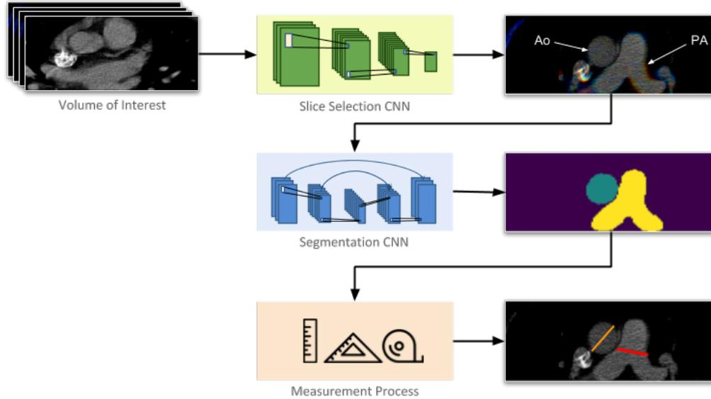
Figure 1: The core system flow with its three consecutive steps of and their respective output. Given the volume of interest, the slice selection CNN is used to select the correct slice for the measurements. The two arteries are labelled in white in the chosen slice, for the reader’s convenience. The chosen slice segmentation map is then generated using a second CNN. Finally, image processing techniques are used to measure the diameters, as shown in orange for the Ao and red for the PA.
